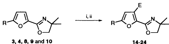
Scheme 6 Reagents and conditions: i, BuLi, THF, -78^{\circ}\text{C} , 0.5 h; ii, electrophile
